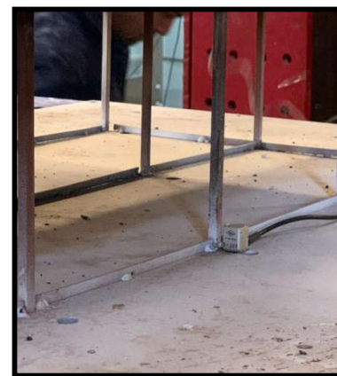
Accelerometer at the bottom
